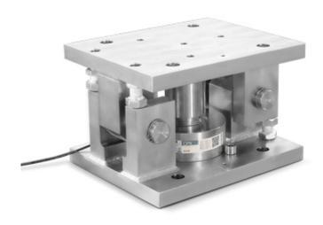
KCP100H is an accessory designed for the correct mounting and operation of CPX series compression <u>load cells</u> below large capacity silos, both horizontal and vertical, in indoor or outdoor environments (up to 100t per support point).
