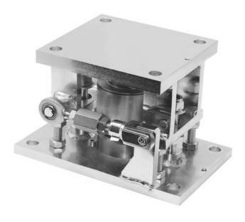
Assembly kits for 40,000 kg RL5426 and RL5426DC series canister <u>load cells</u>. Suitable for weighing silos, hoppers and large capacity tanks.
