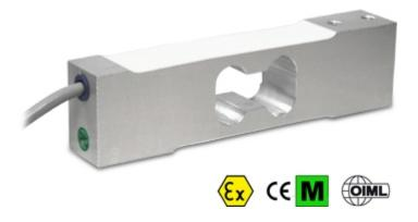
Load cells for off center loads, suitable for example to build CE-M approved scales with a single load cell; maximum platform dimensions of 450x450 mm.
